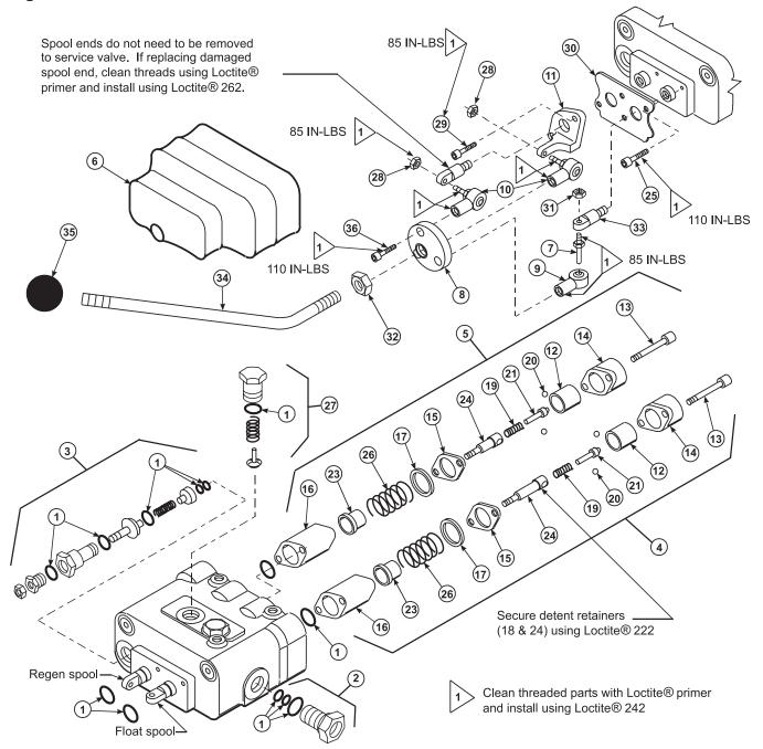
Figure 5 VALVE EQUIPPED WITH LOCKOUT FEATURE
