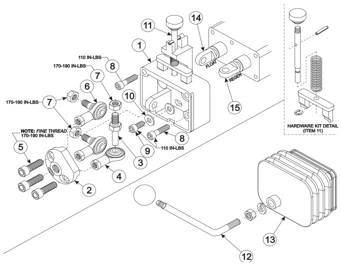
PARTS LIST - JOYSTICK SUB-ASSY WITH DUAL SPOOL LOCK
