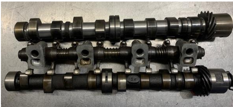
Typical pushrod camshafts (FIAT 600D/850), with rocker shaft setup in centre showing spring-retained rockers and worn tips on end of rocker arm.
