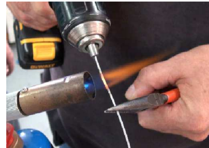
FIGURE 3: TWIST-WELDING PUSH-PULL CABLES
