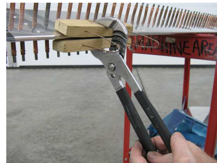
FIGURE 5: TRAILING EDGE TOOL APPLICATION
