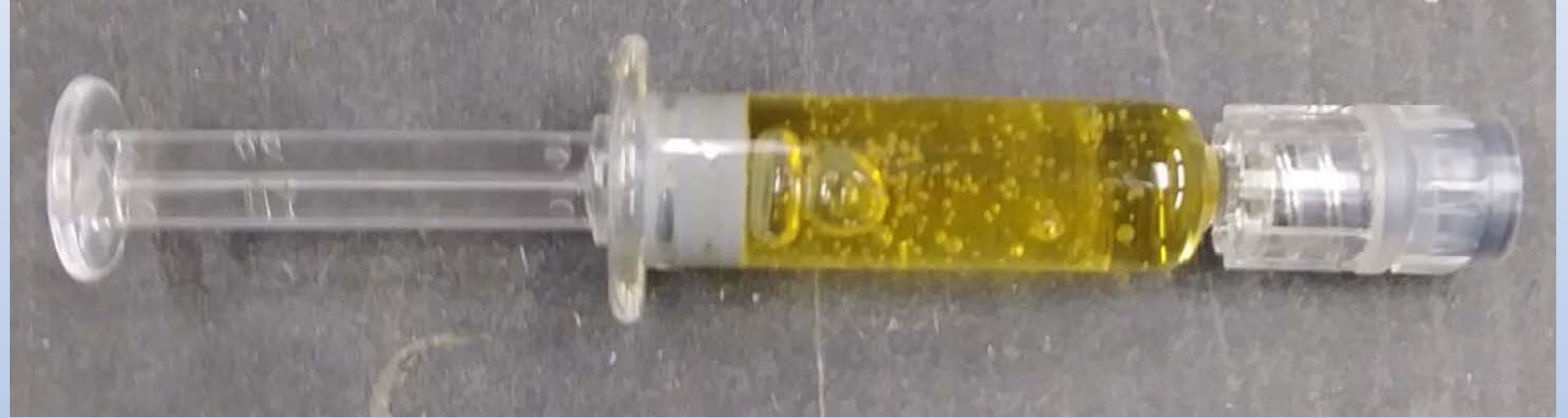
Pine rosin sample in the syringe was analyzed: It contains MCT oil to make it fluid
