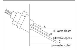
Systems using tap or softened water control water levels electronically using a three-rod probe. The controller responds with the above actions when the water level reaches each rod.
