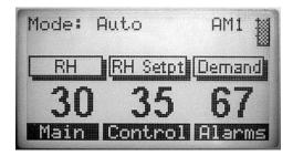
This is the Idle Screen displayed with Vapor-logic3 versions 5.x.x and 7.x.x (systems with multi-tank configuration capability)
