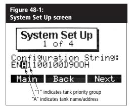
Humidifier tanks ordered as a multi-tank group are configured at the factory. The configuration process includes:
