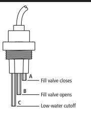
Systems using tap or softened water control water levels electronically using a three-rod probe. The controller responds with the above actions when the water level reaches each rod.
