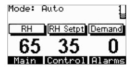
This is the Idle Screen displayed with Vapor-logic3 versions 2.x.x, 3.x.x, 4.x.x and 6.x.x
