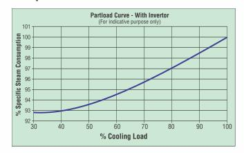
Variable Frequency Drive on absorbent pump for higher reliability, savings in steam & savings in power, during part load operation.
