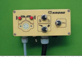
Offered more: The "Medium" monitor informs the operator of the finished bale diameter and starts the tying process automatically or alternatively can be switched to manual mode.
