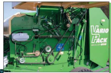
Compaction without complication: Only a few drive chains are needed for the Vario Pack round baler generation. That means the power consumption is kept to a minimum and the machine maintains the highest reliability.
