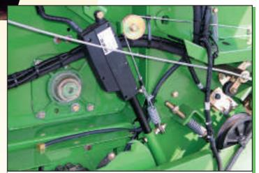
Sure safety: Starting the net-wrap or twine is controlled from a linear motor working in conjunction with the user-friendly monitor. The linear motor tensions a drive belt thus driving the rubber roller for the net or twine feeding it in to the bale chamber.
