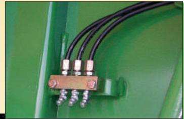
This is comfort: Daily servicing is so easy you can almost rule it out. All the grease nipples are located in a central greasing bank to insure that the awkward ones are not missed out!
