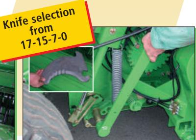
With one turn: The KRONE knife selection of 17 - 15 - 7 - 0 is put into operation! Fast, easy and simple selection of the number of knives required in the chamber. Knife removal is also simple, requiring no tools.
