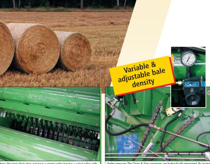
Sure thing: The Vario Pack does not have a starter roller but has a spiral roller with a scraper bar. That ensures fast bale starting and extra bale density with a high core compaction.
