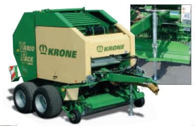
Sure footed: When connecting the round baler there is a robust, fully adjustable parking jack with an integrated folding load step, the jack is easily raised via the step-less spindle.
