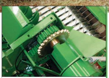
Direct drive: The driveline for the cutting rotor is transmitted via over-dimensioned spur gears that will withstand the highest loads and thus the highest reliability. This is why KRONE round balers handle the toughest conditions and feed uneven swaths with no problem.
