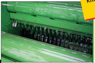
Always the cleanest cut: Up to 17 knives and a theoretical chop length of 64 mm (2.5"). Layout of the knives is in one row and with the smallest of distances between the rotor and the double shearing action guarantees the highest cutting quality.
