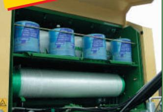
Net and twine in one box: The twine box can also hold one roll of net-wrap and 4 balls of twine. Ideal for differing conditions and customers wishes where in a flash net-wrap can be changed over to twine and vice-versa.
