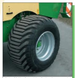
Choice of Rubber: For special applications the correct options must be available to insure the highest productivity. KRONE offers many tire options to fit individual requirements. As an example the 600/50-22.5 tires have many advantages in wet, heavy ground and lower ground compaction – lighter on the soil and the baler.
