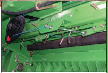
Ideal tying: The stepped pulley applies the twine evenly across the bale surface, thus keeping the crop in a neat and tight roll. The tying stage starts and ends in the middle of the bale meaning no loose twine on the bale edges and a uniform tying process.
