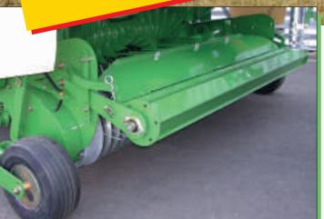
The five rows of galvanised tines lift even the shortest of crops absolutely spotlessly from the ground with automatic chain tensioning, pneumatic feeler wheels and hydraulic lift all standard equipment.
