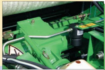
Clean flow: The KRONE round baler even filters the tractor hydraulic oil with the integrated oil filter insuring the oil is always clean. That brings reliability and thus the perfect working conditions without problem.
