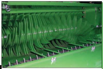
Bon Appétit: The characteristics of the cutting rotor insure an outstanding feed, smooth crop flow and the highest density. The V-formed rotor and double fingers guarantee a high cutting frequency. Better crop feeding...better cut quality...better round bales!
