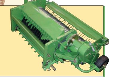
Lift & Cut – continuous smooth feeding: Pick-up and the cutting rotor are a compact unit. The cutting rotor is positioned in the middle of pick-up enabling a smooth and continuous crop flow that is so very important in light and badly structured crops and where the short transfer distance increases the performance.
