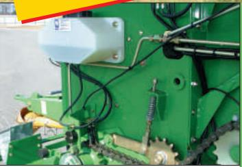
Another plus point for reliability: The Auto-Lube system has an extra large oil reservoir and a heavy-duty eccentric pump. The complete system can be monitored from the tractor seat, by a gauge located at the front that informs the operator of the amount of oil being distributed and thus is reassured that the system is functioning correctly at anytime.
