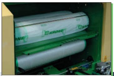
Big enough for the longest day: The twine box is fully protected from the elements and can hold up to 3 rolls of net-wrap. The twine box can handle either 2000 m (??? feet) or 3000 m (??? feet) rolls securely.
