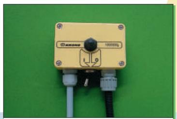
It's very simple: The "Basic" monitor comes as standard equipment with double twining system. When the desired bale diameter is reached the operator presses the button and starts the twine tying.
