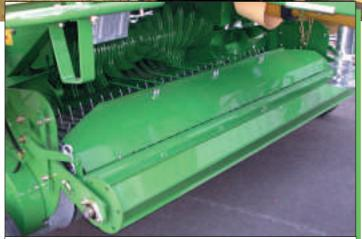
Round and Round: Always a smooth and continuous crop flow through the pickup with this optional crop roller guide turning heavy windrows into higher output. Even without the "MultiCut" cutting rotor KRONE Vario Pack 1500 & 1800 round balers are equipped as standard with a feed rotor between the pick-up and bale chamber thus insuring a fast and direct feed into the huge bale chamber entrance.
