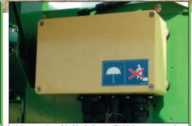
Job Computer – heart of the "Comfort" monitor: The Job Computer receives all electrical impulses from the sensors and then transfers them to the monitor. It also transfers commands from the monitor to the sensors on the baler, for example; setting the automatic tying on.
