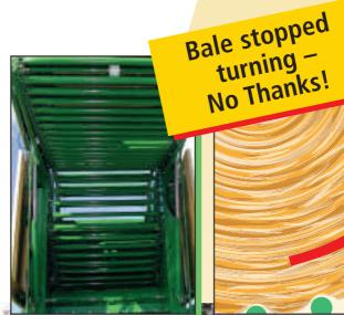
Distinctively KRONE: Two continuously rotating Chain and Slat conveyors make up the Vario Pack bringing reliability, durability and long life, not forgetting also that it delivers the tightest, highest quality bales in it's class. No bales at a standstill – guaranteed rotation: The grip effect of the slats pulls the material into and around the bale chamber keeping it turning, regardless of the conditions and even in dry straw. Just one of the benefits of a Chain & Slat conveyor.
