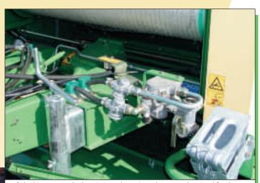
Safe braking: As standard equipment the Vario Pack 1800 and optional for the 1500 is fitted with compressed air brakes. For both machines as an export variant hydraulic brakes can be fitted, to assure safe road transport at speeds of up to 40km/h (25 mph).
