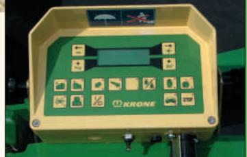
Operator Comfort: The "Comfort" monitor is renowned for it's clear, functional and simple operation. The operator is kept informed of all functions through both visual and acoustic alarms that intervene when necessary.
