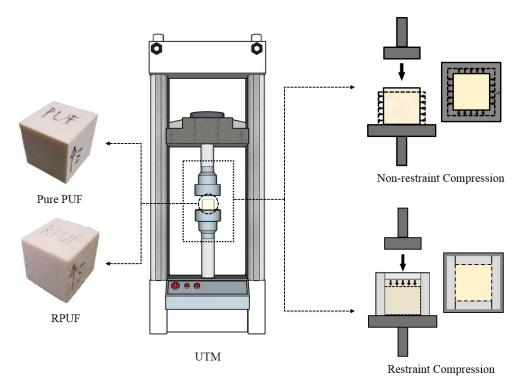
Figure 4. Mimetic diagram of test specimen and equipment.
