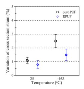
**Figure 9.** Variation in the cross-section of the rigid PUF specimen according to the compressive test method.
