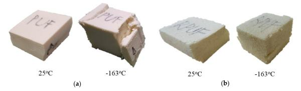
**Figure 5.** Shape of the specimens after the compressive test according to the temperature under the standard of the conventional compressive test: (**a**) PUF, (**b**) reinforced polyurethane foam (RPUF).
