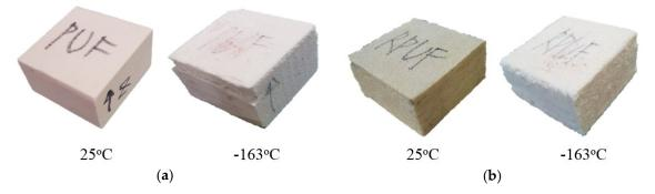
**Figure 7.** Shape of the specimens after the compressive test according to the temperature under restraint of the suggested compressive test: (**a**) pure PUF, (**b**) RPUF.
