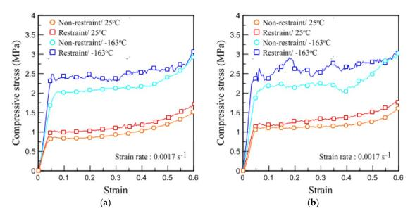
**Figure 10.** Compressive stress–strain curves for (**a**) pure PUF and (**b**) RPUF according to the environmental conditions of the restraint system.
