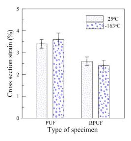
Figure 6. Cross-sectional strain of the rigid PUF after the conventional compressive test.
