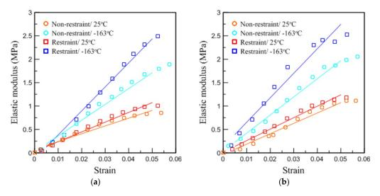
Figure 11. Dependences of the elastic modulus on restraint for (a) pure PUF and (b) RPUF.
