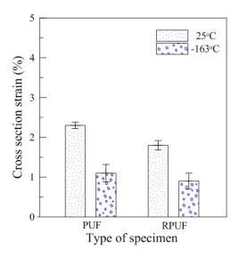
Figure 8. Cross-sectional strain of the rigid PUF after the restraint compressive test.
