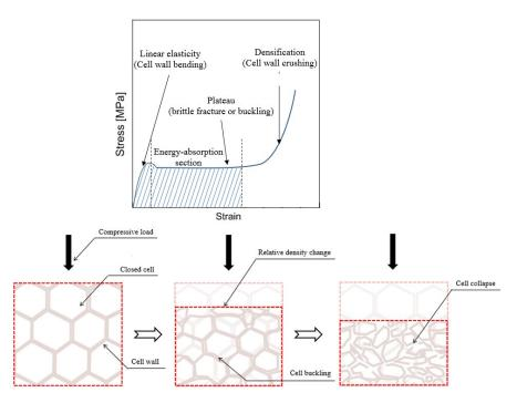
Figure 3. Mechanical behavioral characteristics of rigid PUF under a compressed load.
