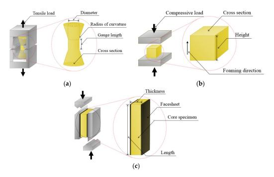
**Figure 2.** Evaluation of the mechanical performance of rigid PUF according to international standards: (a) tensile, (b) compression, and (c) shear test methods.
