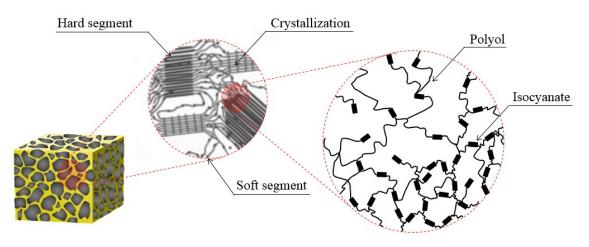
Figure 1. Domain structure that forms the inside the polyurethane foam (PUF).
