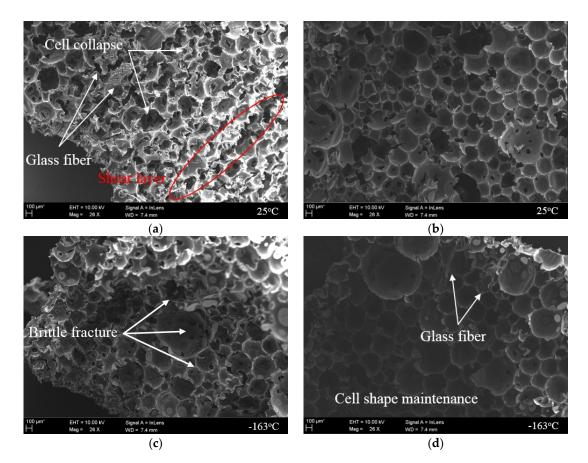
**Figure 13.** Microstructure inside the RPUF after the compressive tests according to the restraint condition. (**a**) non-restraint at 25 °C; (**b**) restraint at 25 °C; (**c**) non-restraint at -163 °C; (**d**) restraint at -163 °C
