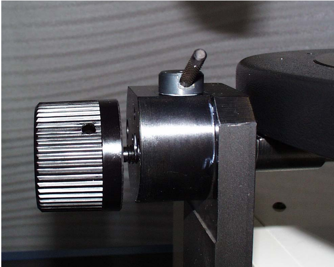
DISTORTION FREE DISK BRAKE WITH MANUAL INDEXING RELEASE
