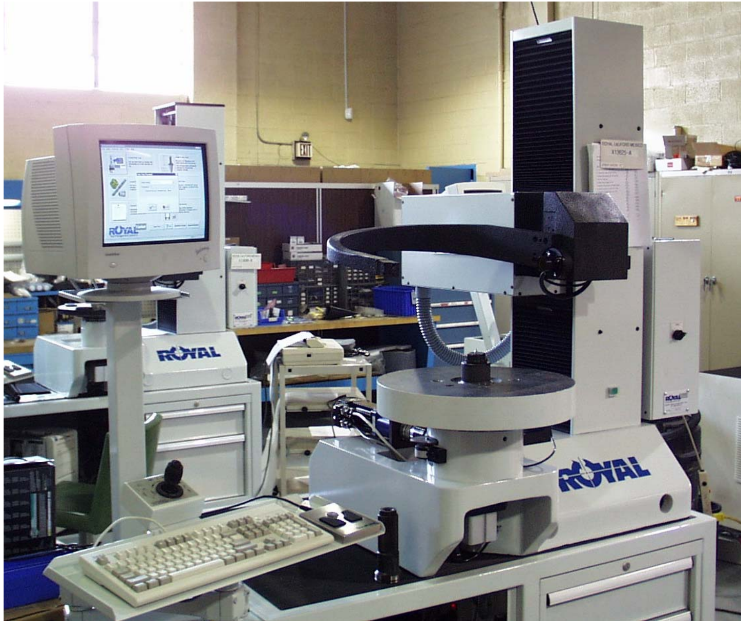
3FVP 620/190 THIRD AXIS GAUGE WITH GRANITE TABLE
