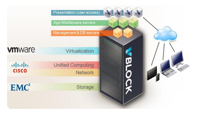
For each of these layers, physical and logical components need to be sized to meet customer requirement (Workload, Bandwidth, and Storage) by considering best practices and overhead while provisioning compute, network, and storage resources.
