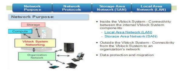
VBlock System servers have no storage and their OS files are stored on storage devices. Instead of separate IP and SAN switches, VBlock systems can be built with Cisco Unified Switch. A unified switch can perform tasks associated with both IP and Fibre Channel networks. However, a separate LAN and SAN switch would have more ports than a Unified switch. Hence, we have two options to consider for Network in VBlock Systems:
