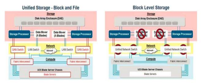
Storage should be sized to handle workload and capacity of the applications for the VBlock Systems. Workload and Capacity requirement decides the optimal storage system for a VBlock. Storage system decides the VBlock system model. Below table can be used to understand type of hardware used currently across all 3 layers in a VBlock.
