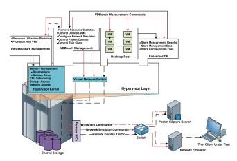
Fig. 2. Components of VDBench and data flows
