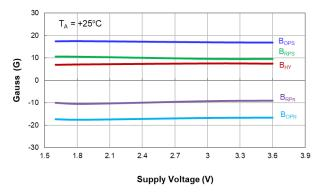
Switch Points  $B_{\text{OPS}}$  and  $B_{\text{RPS}}$  vs Supply Voltage
