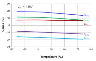
Switch Points  $\mathbf{B}_{\text{OPS}}$  and  $\mathbf{B}_{\text{RPS}}$  vs Temperature
