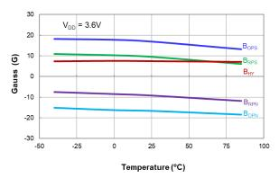
Switch Points  $\mathbf{B}_{\text{OPS}}$  and  $\mathbf{B}_{\text{RPS}}$  vs Temperature
