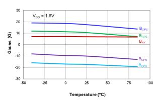
Switch Points  $B_{\text{OPS}}$  and  $B_{\text{RPS}}$  vs Temperature
