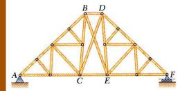
• Truss contains a *redundant member* and is *statically indeterminate*.
