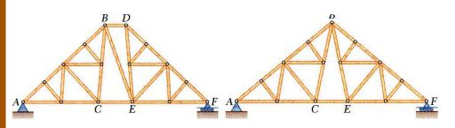
• *Compound trusses* are statically determinant, rigid, and completely constrained.
