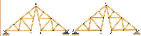
Necessary but insufficient condition for a compound truss to be statically determinant, rigid, and completely constrained,
