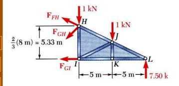
• Apply the conditions for static equilibrium to determine the desired member forces.
