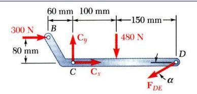
$$\sum M_C = 0 = (F_{DE} \sin \alpha)(250 \text{ mm}) + (300 \text{ N})(60 \text{ mm}) + (480 \text{ N})(100 \text{ mm})$$
