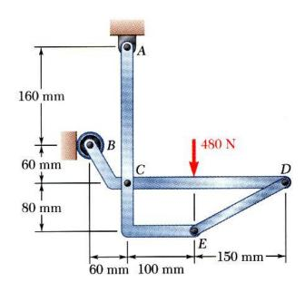
Members *ACE* and *BCD* are connected by a pin at *C* and by the link *DE*. For the loading shown, determine the force in link *DE* and the components of the force exerted at *C* on member *BCD*.
