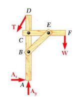
• A free body diagram of the complete frame is used to determine the external forces acting on the frame.
