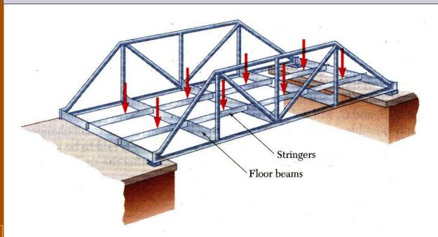
Members of a truss are slender and not capable of supporting large lateral loads. Loads must be applied at the joints.
