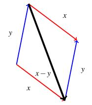
Finally, we note that the parallelogram can be used to simulaneously illustrate vector addition and subtraction:
