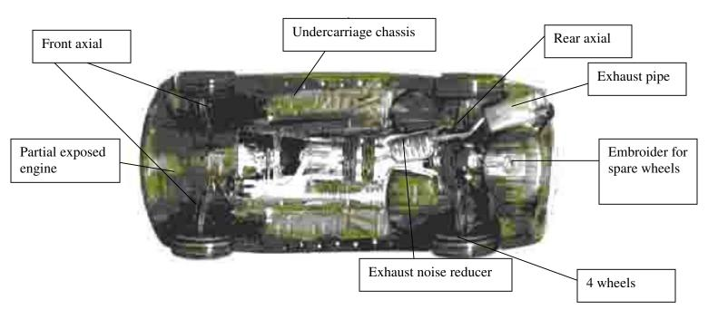
Figure 4: Component of typical vehicle undercarriage
