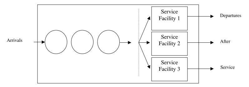
Figure 28: Multi-channel, single- phase system
