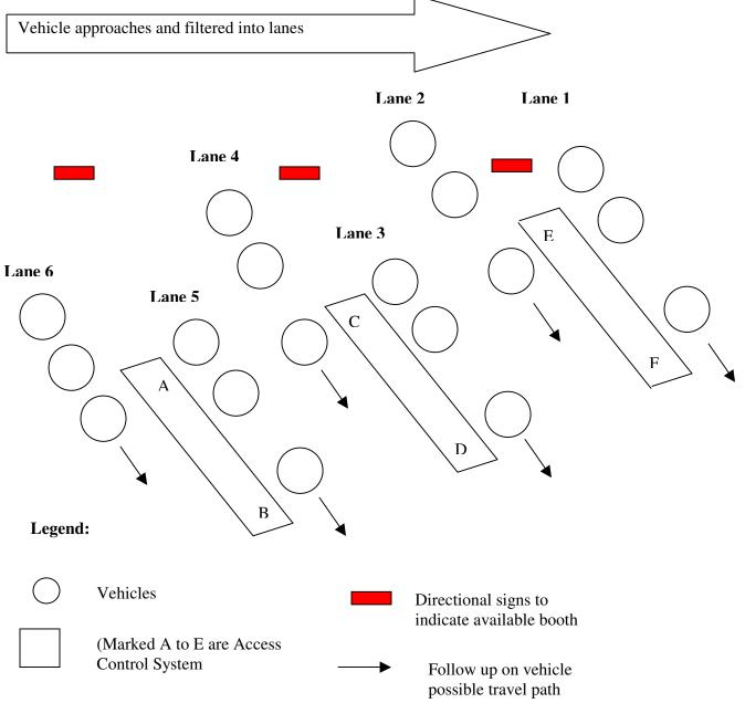
Figure 31: 3 accessing platform, 6 lanes access control
