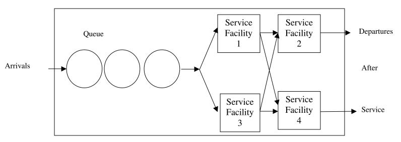
Figure 29: Multi channel, multiphase system
