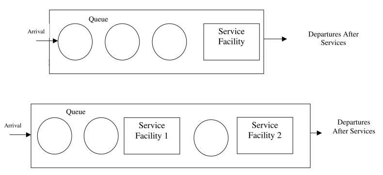
Figure 27: Single channel, multiphase system
