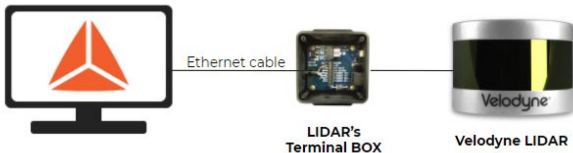
Image 2: Standalone system configuration
