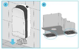
Air Filters: To be checked often and cleaned if necessary.
