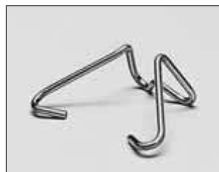
1 1/2" DRYWALL FURRING CHANNEL CLIP Attaches Screw Furring Channel to 1 1/2" cold rolled steel channel.
