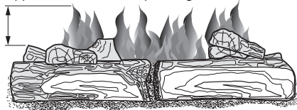
Figure 33 - Correct Burner Flame Pattern
