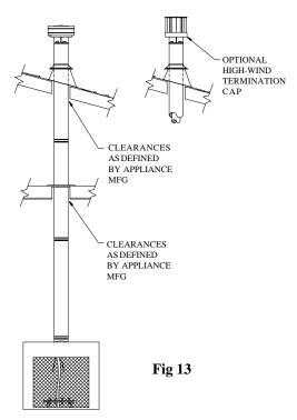
penetrate the ceiling. Drill a small hole at this point. Next, drop a plumb bob from the roof to the hole previously drilled in the ceiling, and mark the spot where the vent will penetrate the roof. Determine if ceiling joists, roof rafters, or other framing will obstruct the venting system. You may wish to relocate the appliance, or to offset, to avoid cutting loadbearing members.
