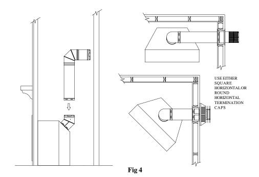
twist-locked and rotated to face the wall termination, with final positioning of the vent pipe assembly determined by the mounting orientation of the appliance adaptor onto the fireplace. Figure 4 shows some of the possible vent pathway options. Consult the appliance manufacturer for any restrictions.
