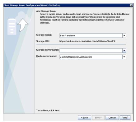
Provider and access details are used to map the cloud storage settings to NetBackup storage settings. The cloud storage region is mapped to the NetBackup storage server. All the backups that are targeted to the NetBackup storage server use the cloud storage region to which it is mapped.
