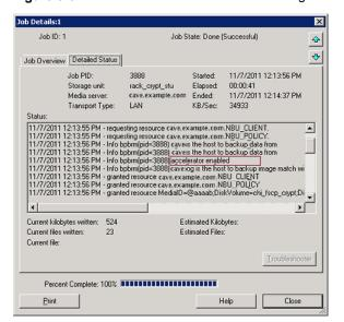
Figure 3-5 Confirm Accelerator used during backup
