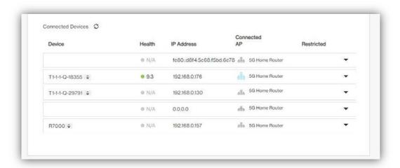
Select the arrow icon "v"on the right that correspond to a connected device, and related information and settings for the device will be displayed, including its IPv6 address, whether to delete the device, block the device, or reserve DHCP IP.
