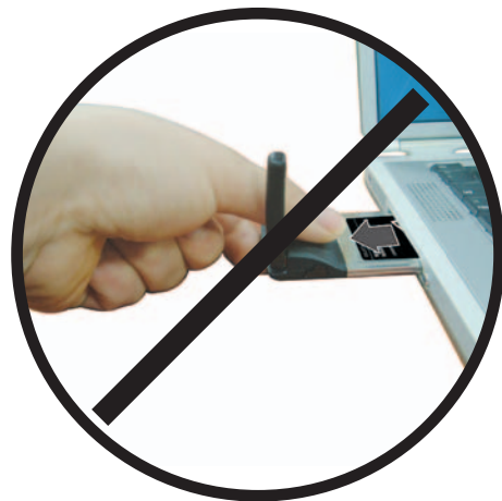
Do not handle or remove the PC Card by pulling on the antenna.
