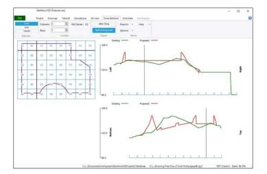
The project boundary with the grid lines are displayed on the left side of the **Cross Sections** tab. As noted previously, the grid spacing is set at the **Calculations** tab. The top left side of the Cross Sections toolbar, has three Selections: **Grid**, **Line** and **Trench**.
