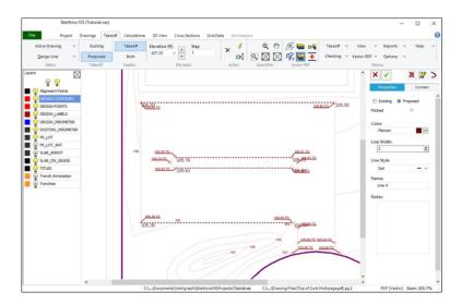
When recording design lines with the **Options** | **Show Properties/Elevation Dialog** checked, the elevation of the points contained in a design line may be calculated based on a slope by checking the **Pitched** check box. After clicking the **Pitched** check box, enter either a rise and run value or a percentage. For lines the slope downwards, the slope % or rise value will be negative. This tool is helpful in determining the end point elevations of a line with a constant slope.
