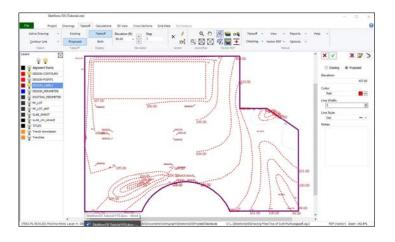
Like the existing contour lines, simply set the elevation and then click on a point in the proposed contour line to takeoff the entire line. When done with the contour lines, turn on all layers by clicking the yellow lightbulb at the very top of the layers list on the left side of the window.
