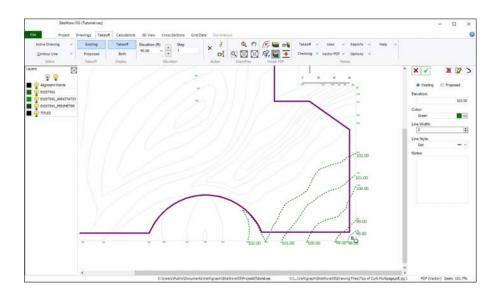
Please remember, zooming is best done using the scroll wheel on the mouse and moving around the drawing (i.e. panning) is performed by holding the keyboard **Ctrl** key while dragging the mouse. Practice moving around, panning, changing elevations and recording contour lines.
