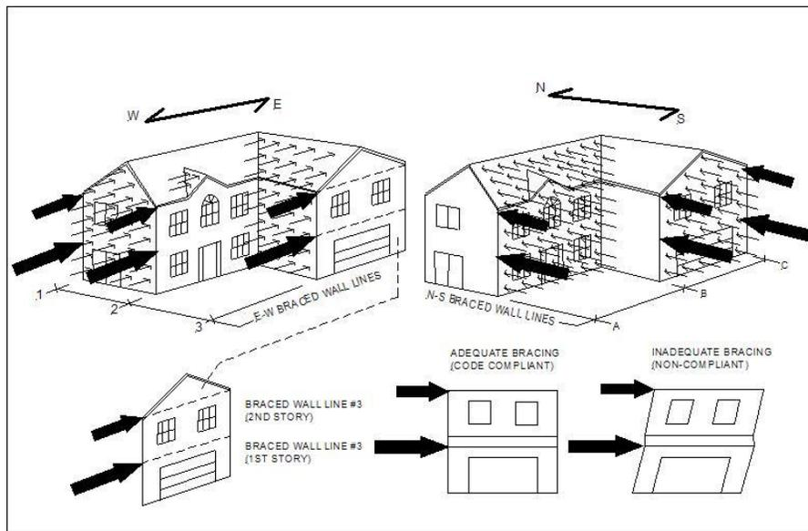
**Figure 1: Wall Bracing and Racking Forces**
