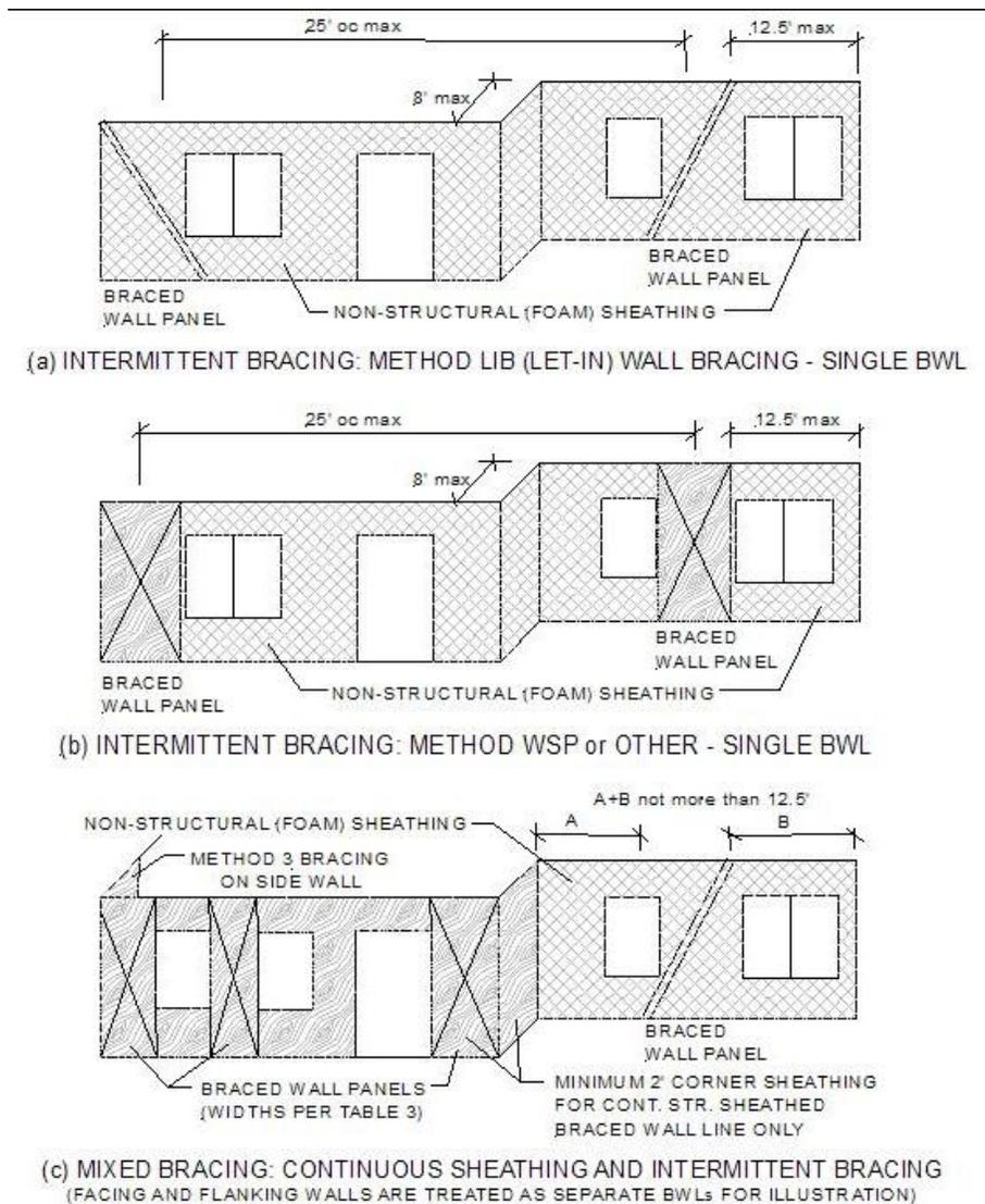
**Figure 20: Illustration of Bracing Methods with Foam Sheathing**
