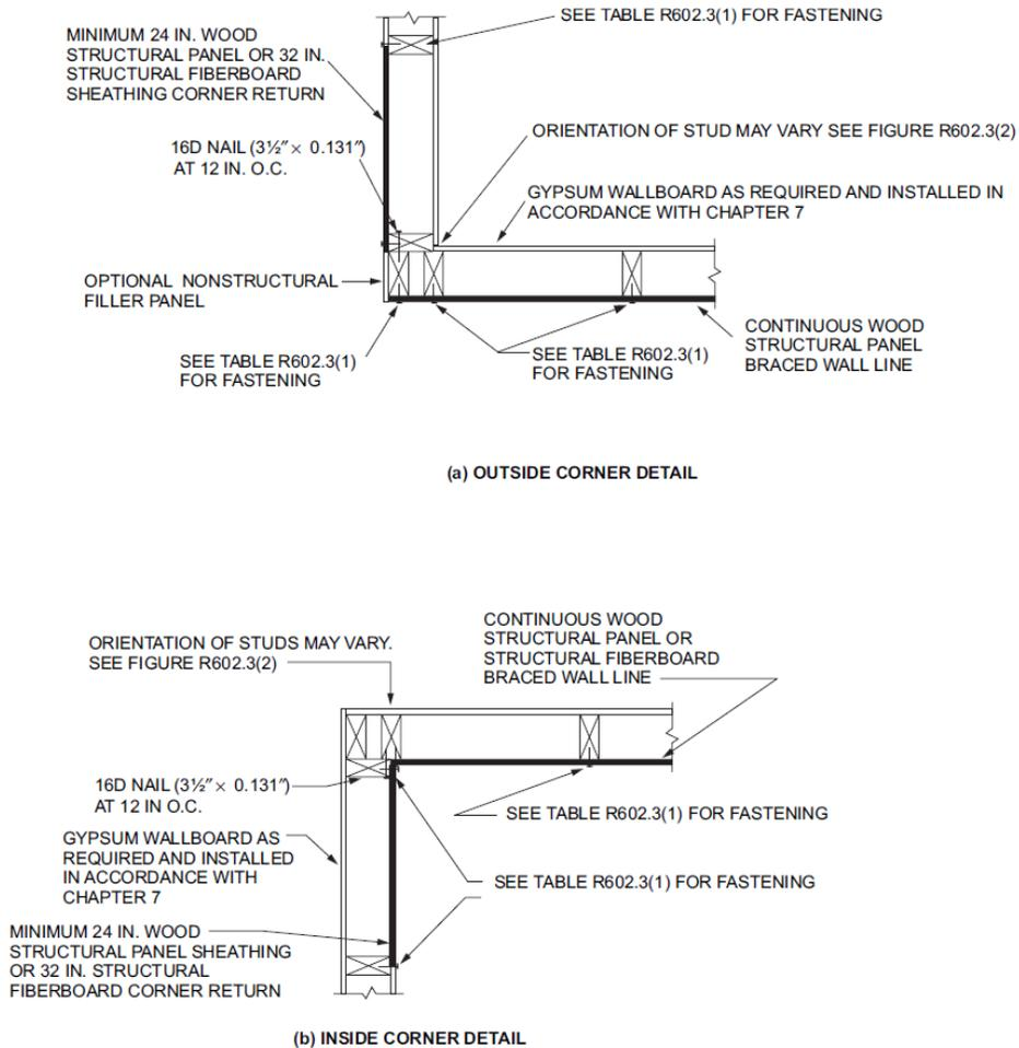
**Figure 11: Corner Framing for Continuous Structural Sheathing**
