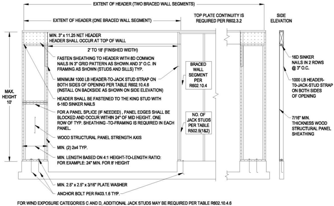
**Figure 7: Method PFG Portal Frame at Garage Door Openings**
