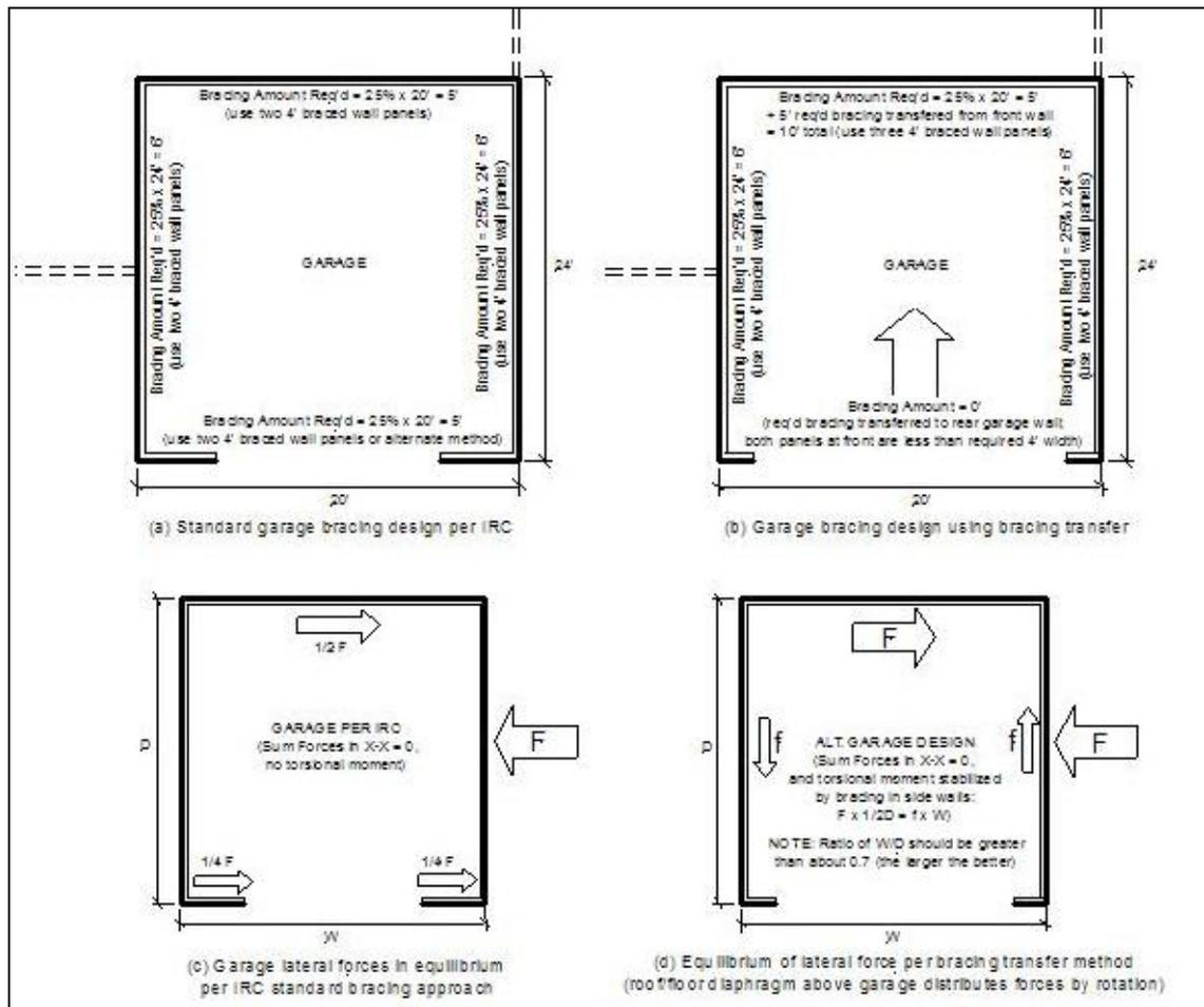
**Figure 18: Bracing Transfer**
