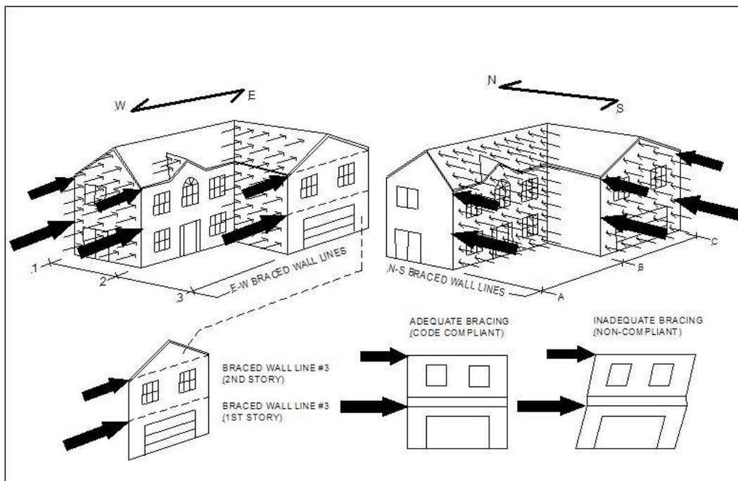
**Figure 17: Example house plan for bracing length calculation**
