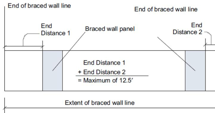
Braced wall panel shall be permitted to be located away from the end of a braced wall line, provided the total end distance from each end to the nearest braced wall panel does not exceed 12.5'. If braced wall panel is located at the end of the braced wall line, then end distance is 0'.
