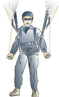
Pulling hard down on the control handles to 'flare' the glider for landing
