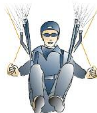
Lowering the control handles to decrease airspeed
