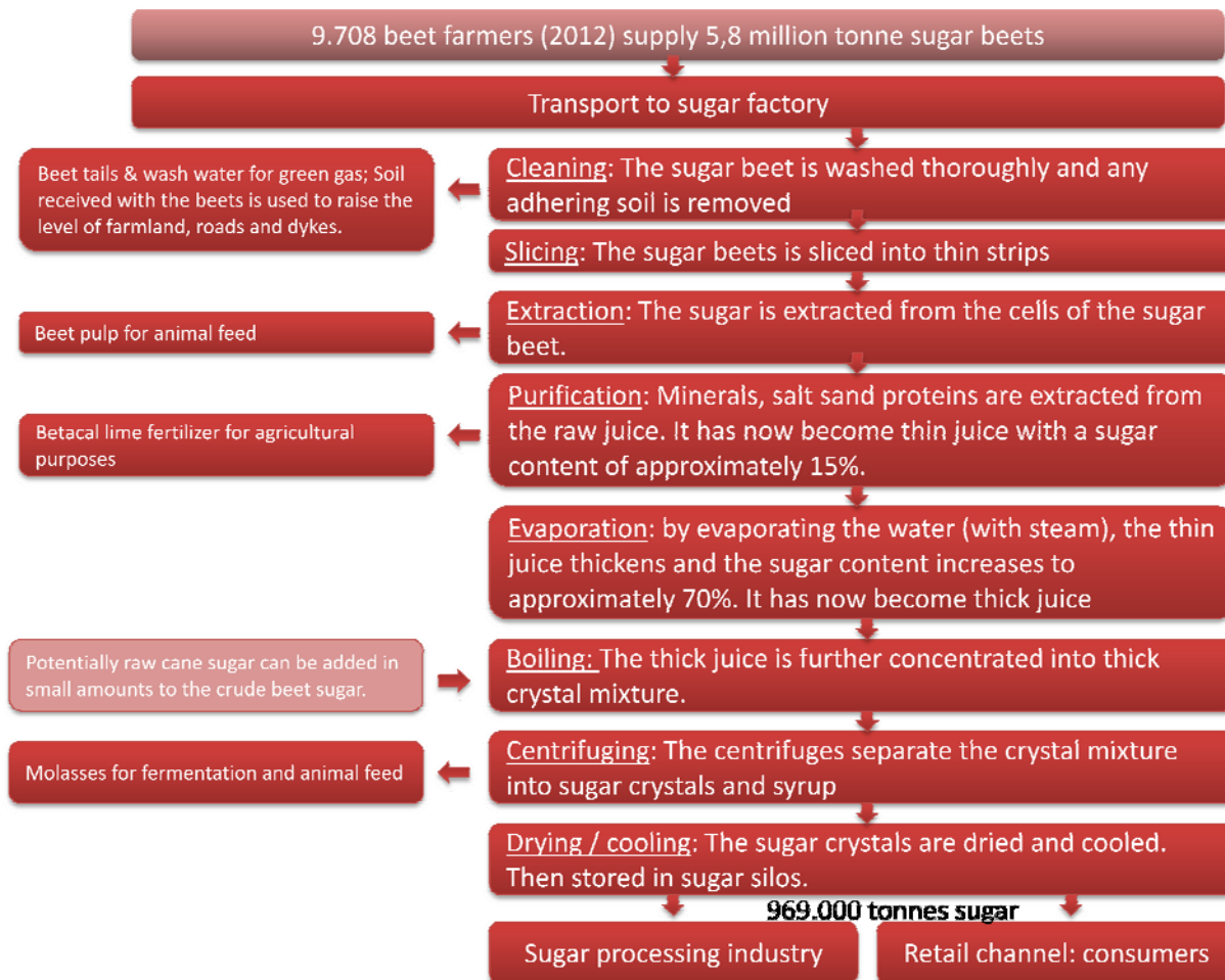
Figure 3.1 From sugar beet to white sugar
