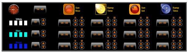
Each color channel can be modified also by changing the times of 'Sun Rise' and 'Sun Set'. Additionally you can set the ramps, so that during the dimming times different color scenes are created.
