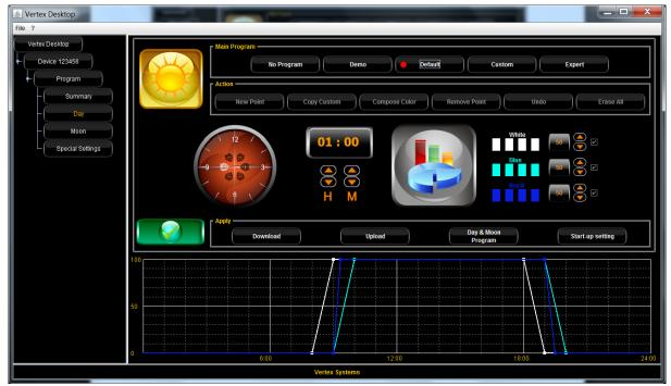
The program Default includes a standard program, which is factory made. No modifications are possible.
