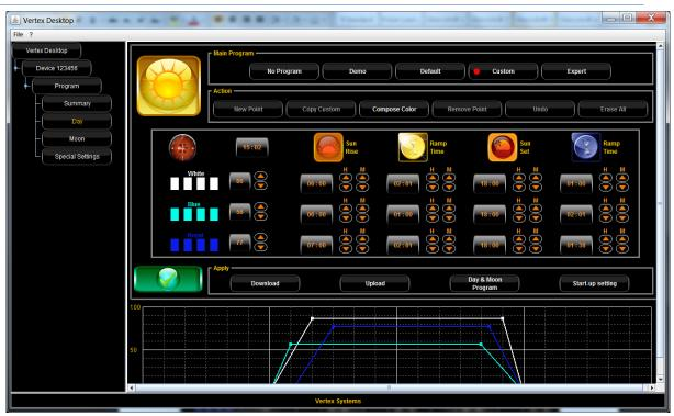
The program Custom is a template, where all the channels can be parameterized by intensity, rise- and dawn timings separately.
