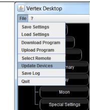
After installing the V-stick start the software. To search for new devices in reachable distance around the V-Stick chose FILE – UPDATE DEVICES. On startup all 'accepted' devices are displayed in the tree structure automatically. Watch out for Accept Queries on the device on select 'Update Devices' in the 'Vertex Desktop'.
