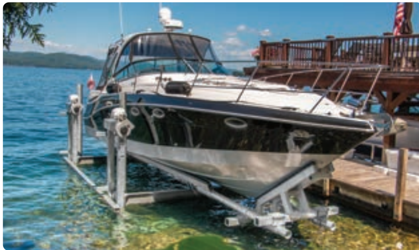
Above: 24,000 lb. capacity Ultimate Lift with custom front end bow stop & optional oil bath drives.
