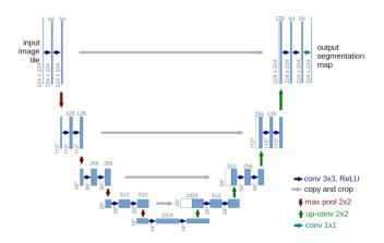
**Figure 1**: U-Net architecture (10) that we use in our preliminary work. Shown here are dimensions of our images in each layer and the number of convolutional and transposed convolutions per layer.
