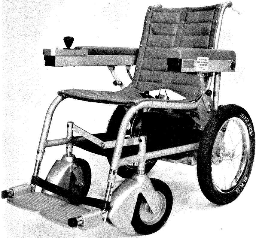
FIGURE 11.—Sun Industries Curb-Climbing Electric Wheelchair.
