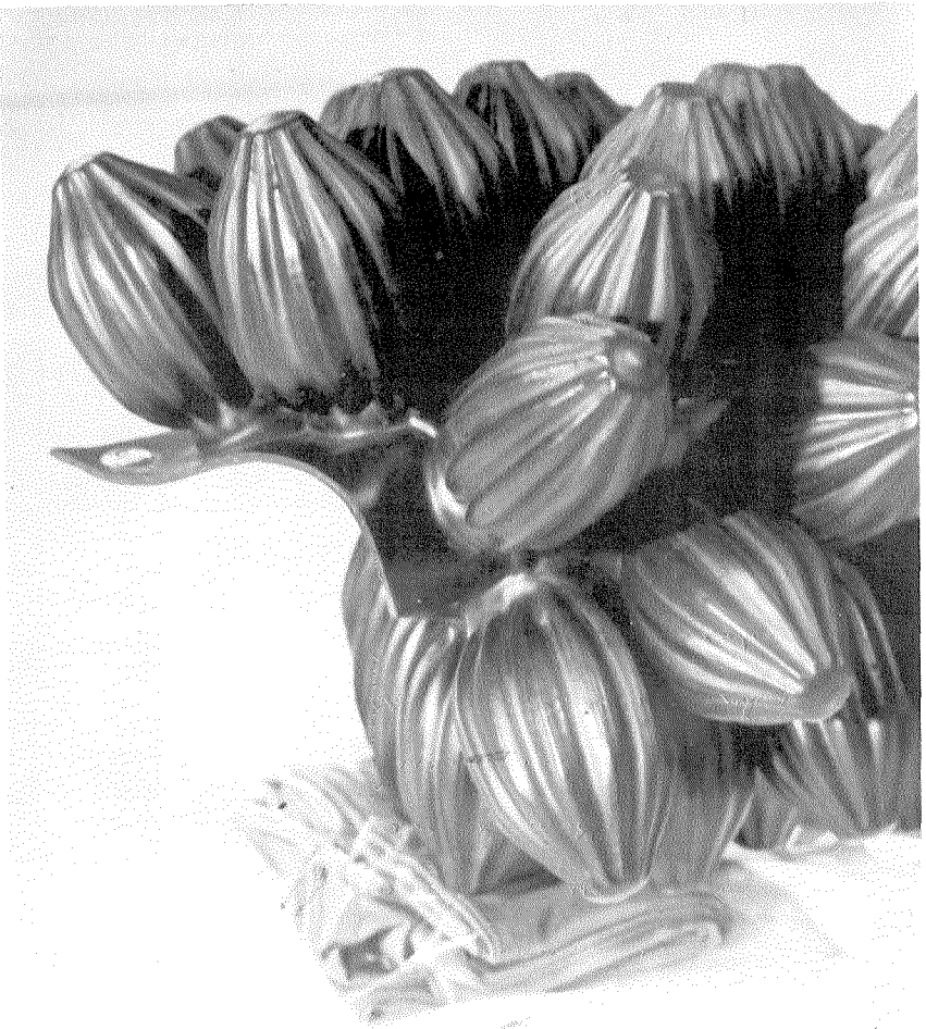
FIGURE 22.—Balloon elements shown attached to neoprene rubber base.
