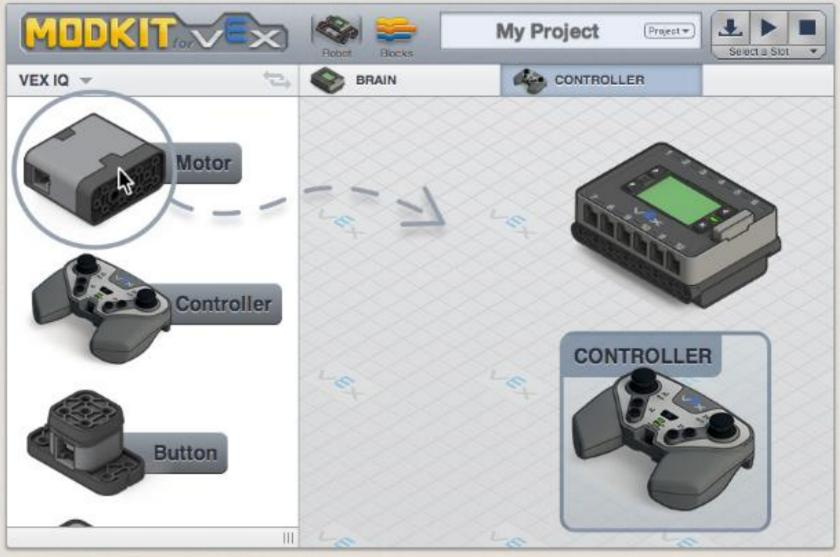
In Robot View, drag & drop a Motor and Controller to the Robot Pad.
