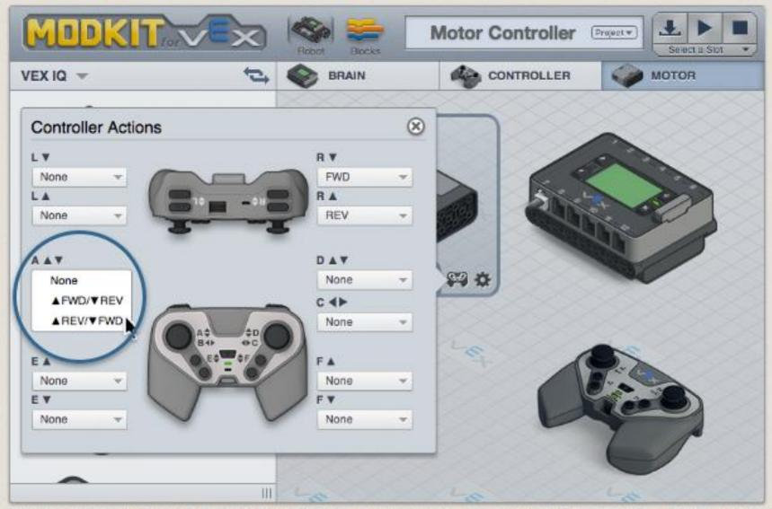
Select actions for the R▲ and R▼ buttons and then set the Joystick A action to ▲ FWD / ▼ REV
