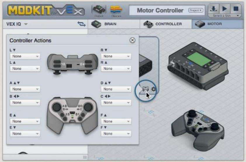
Then click the Controller Actions button next to the port menu to open the Controller Actions window.
