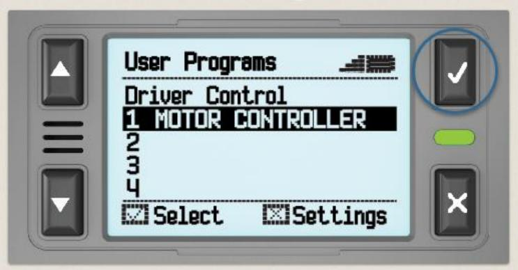
Select the program in the slot number you chose and run it. Both the joystick and controller should control your motor now.
