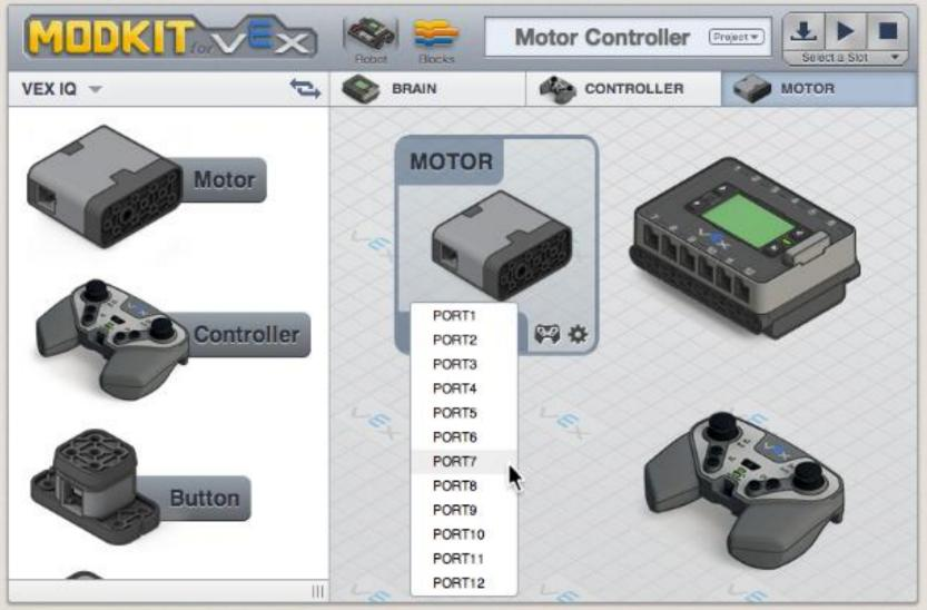
Select port 7 for the Motor. Make sure you've plugged the motor into port 7 on your Robot Brain.
