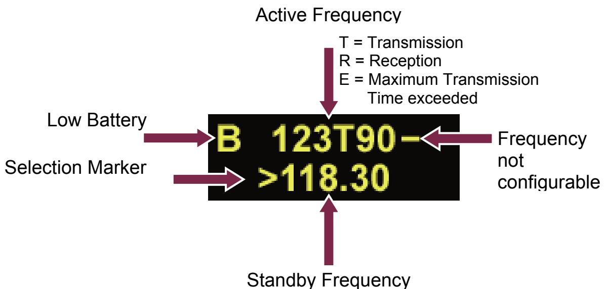
The display of the ATR500 consists of two rows. Apart from the INIT-Menu (see 2.8.1) the upper row always shows the active frequency.
