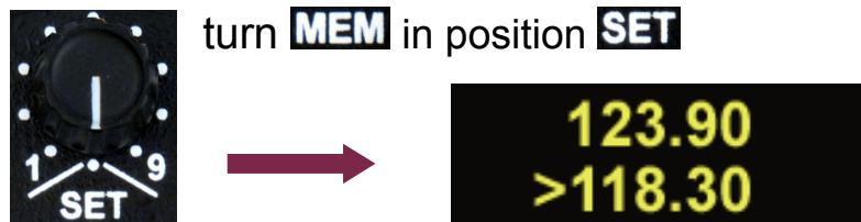
With the input area (MHz or kHz) can be selected:
