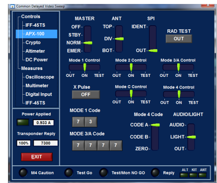
VirtualPanel software example for manual control of LRU
