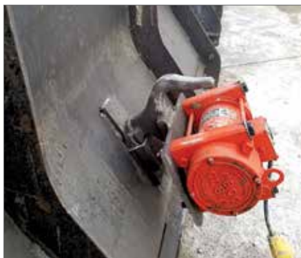
The wider UWF-3 Heavy Duty Wedge Bracket is used for stronger forces.
