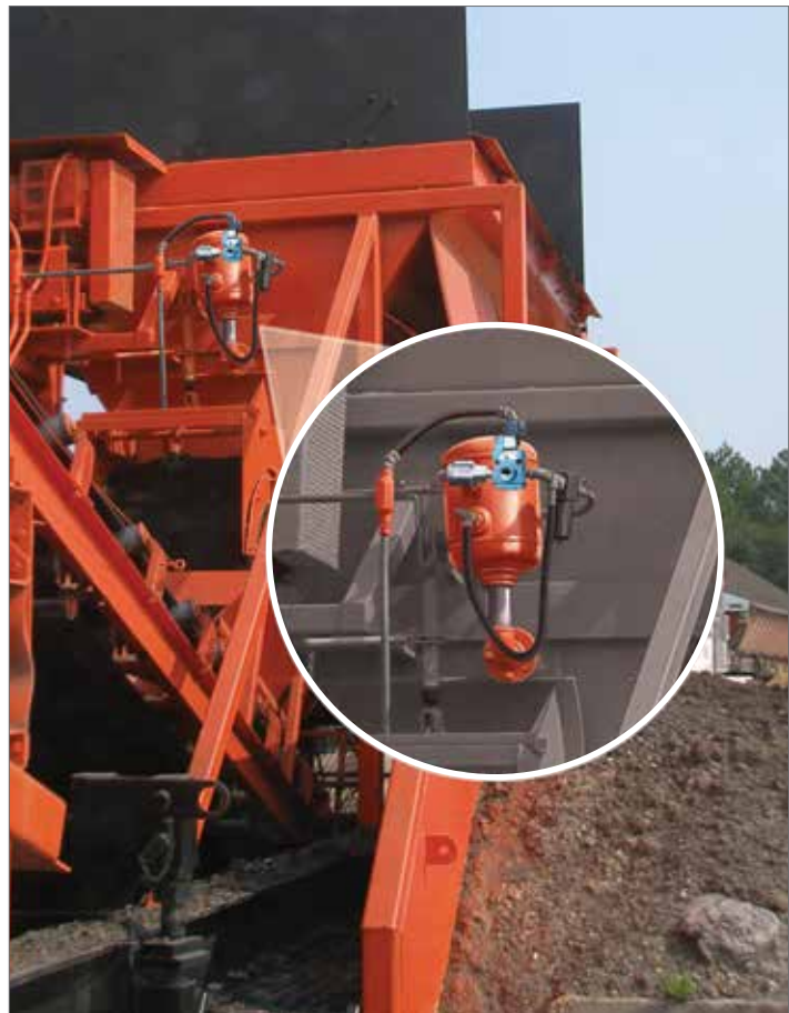
Right: A VIBCO Air Cannon (page 66-67) shown in the white circle, helps to maintain an even flow on the conveyor.
