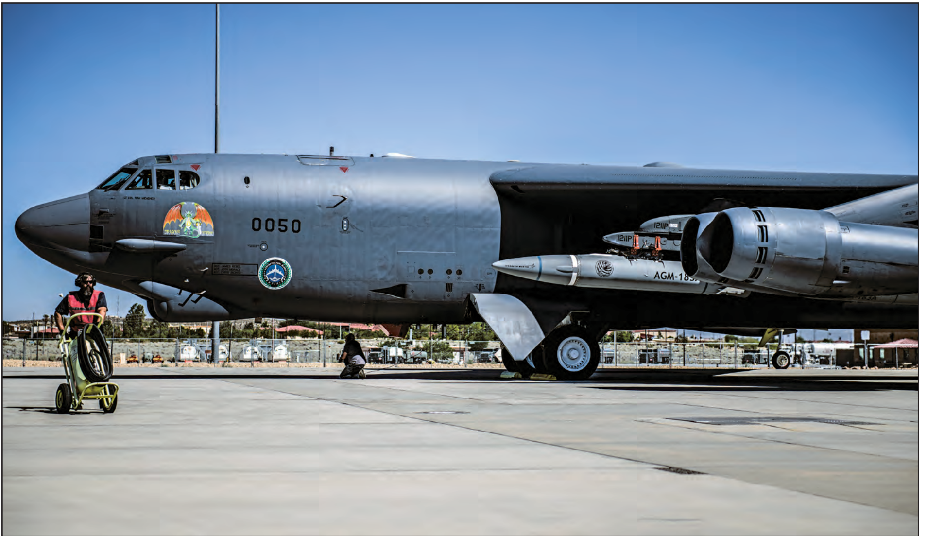
A B-52H Stratofortress assigned to the 419th Flight Test Squadron is undergoes pre-flight procedures at Edwards Air Force Base, Calif., Aug. 8. The aircraft conducted a captive-carry flight test of the AGM-183A Air-launched Rapid Response Weapon Instrumented Measurement Vehicle 2 at the Point Mugu Sea Range off the Southern California coast. (Air Force photo by Giancarlo Casem)
