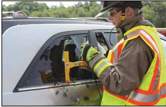
Figure 8.10 A glass hammer is sometimes used to remove vehicle glass.
