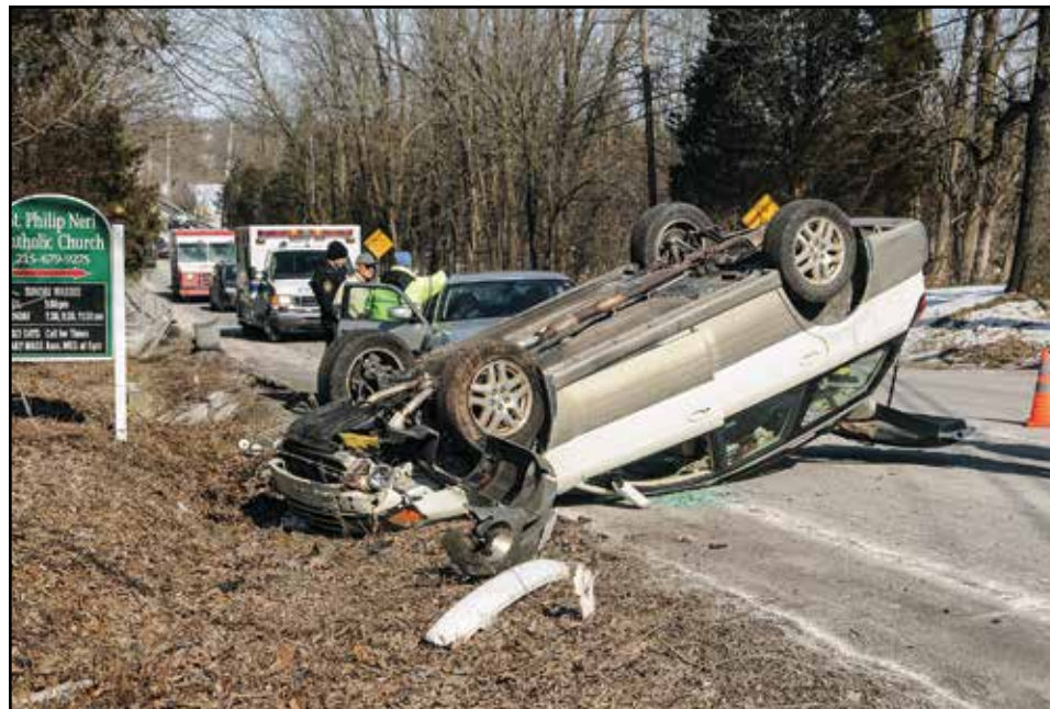
Figure 8.3 Rollover accidents can become more serious if the roof collapses. Courtesy of Bob Esposito.
