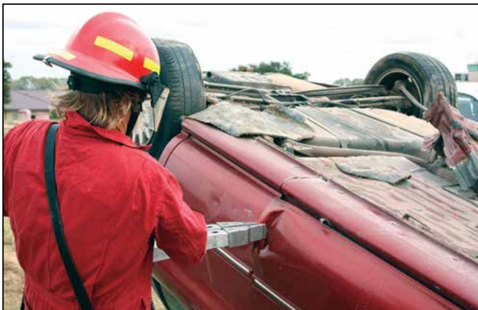
Figure 8.13 Hydraulic spreaders being used to create a purchase point on a rear door of a passenger vehicle.
