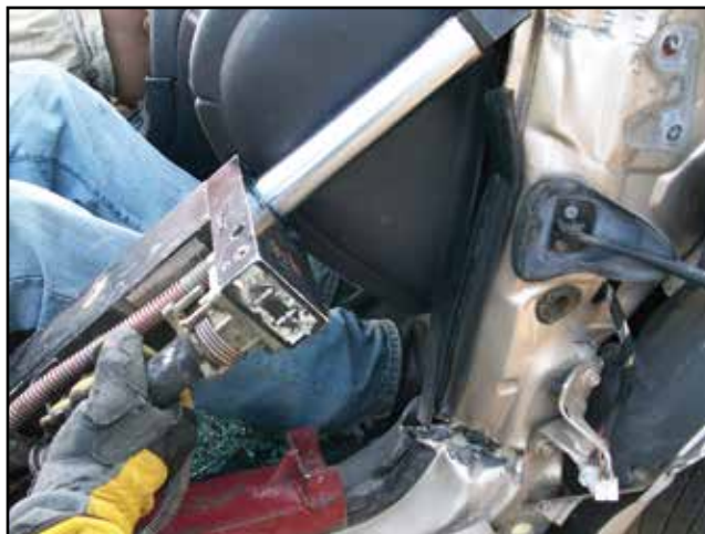
Figure 8.17 A hydraulic ram being used to roll a dashboard. Courtesy of Alan Braun, University of Missouri Fire and Rescue Training Institute.
