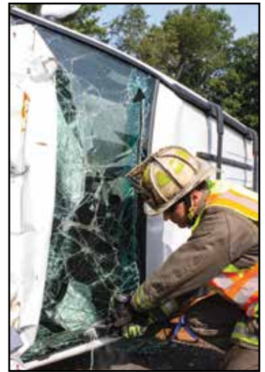
Figure 8.8 A rescuer removing a windshield on a side resting vehicle.
