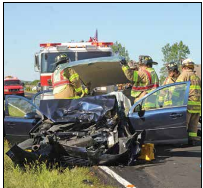
Figure 8.16 Rescuers removing a roof from a passenger vehicle to access the victim. Courtesy of Bob Esposito.
