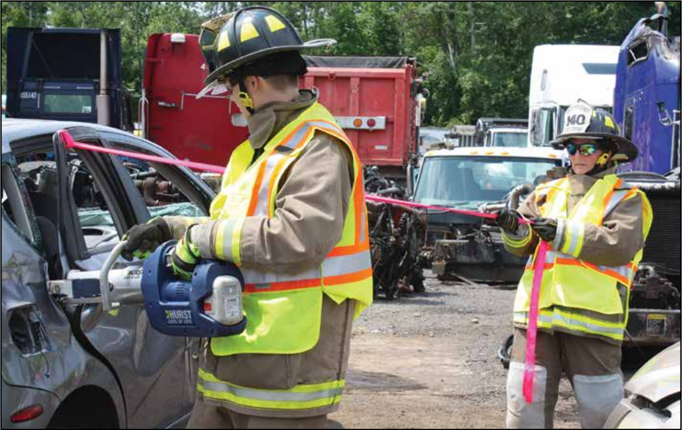
Figure 8.12 Webbing can be attached to a door to maintain control of the door while it is being opened or removed.
