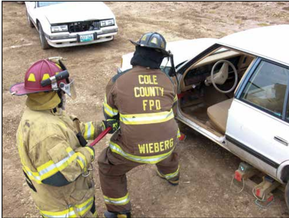
Figure 8.19 Rescuers can use webbing to pull vehicle door pedals away from a victim's feet. Courtesy of Alan Braun, University of Missouri Fire and Rescue Training Institute.
