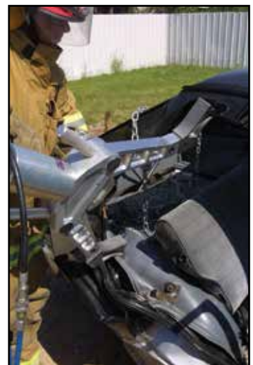
Figure 8.11 A rescuer performing a third door conversion.
