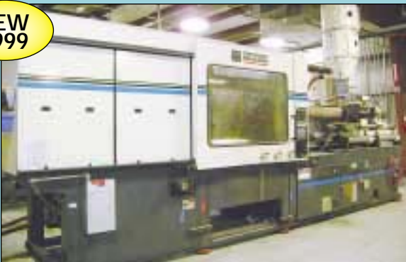
440 Ton X 54 Oz. Cincinnati Milacron Model VT440-54 Horizontal Toggle Clamp Injection Molding Machine
