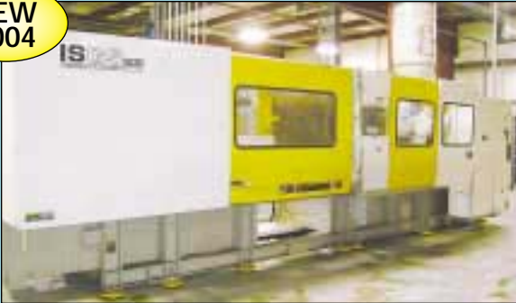
500 Ton X 48 Oz. Toshiba Model ISGS500WV21-27 Horizontal Hydraulic Clamp Injection Molding Machine
