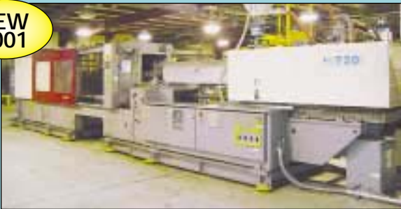
720 Ton X 162 Oz. Goldstar Model 720N Horizontal Hydraulic Clamp Injection Molding Machine
