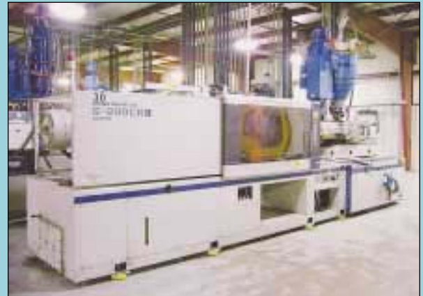
280 Ton X 27 Oz. Shinwa Seki Model S280-CNII-PU28-65 Horizontal Hydraulic Clamp Injection Molding Machine
