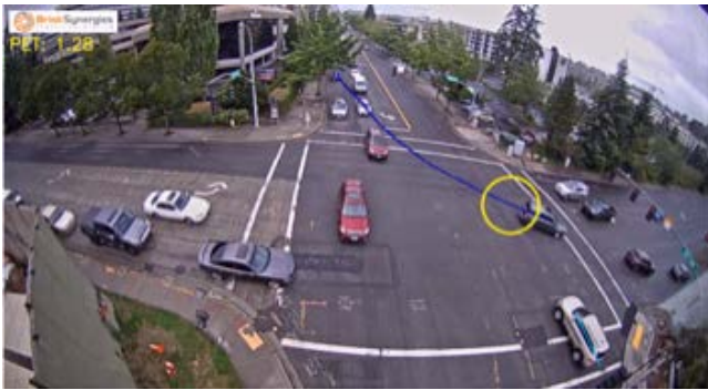
Figure 4.3 – Southbound left turning and northbound through driver conflict at 112th Ave & Main St
