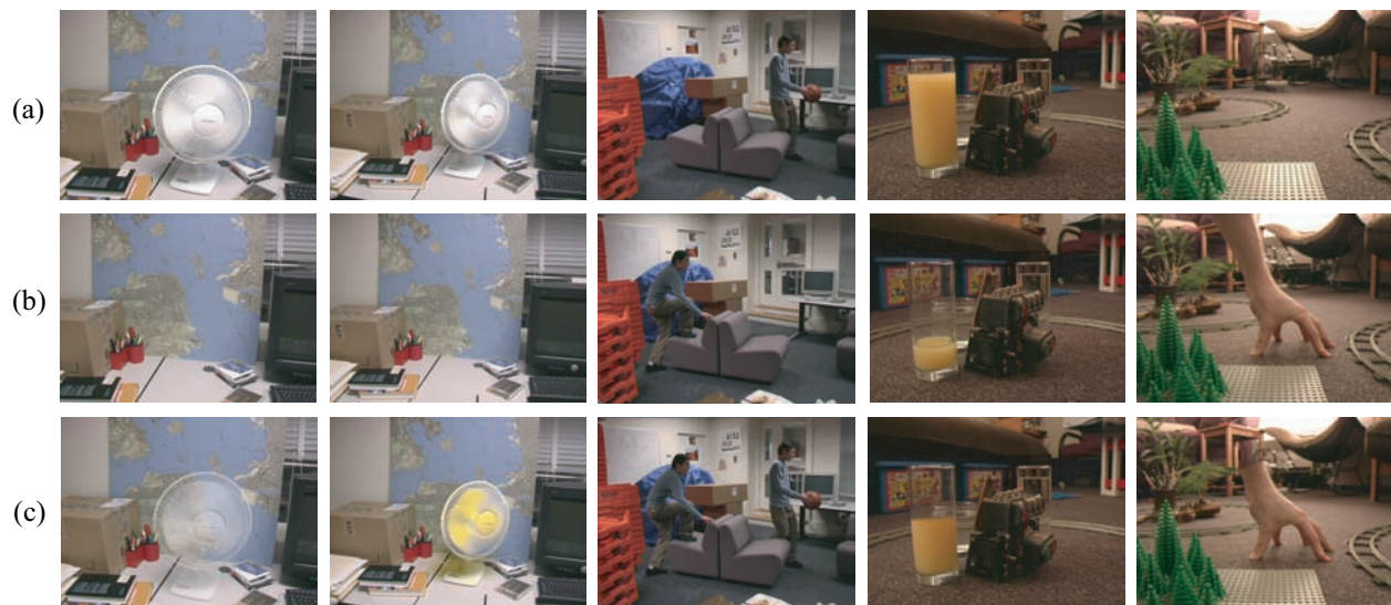
Figure 9: This figure shows primary frames (a) , secondary frames (b) , and various composites (c) . From left to right: (1) a transparent fan created by blending the two frames, (2) color manipulated according to a difference matte, (3) cloning a person by compositing the left half of one image with right half of another, (4) changing the amount of orange juice using a horizontal compositing line, and (5) a dismembered hand with a key-framed compositing line. None of the composites require per-frame manual rotoscoping.
