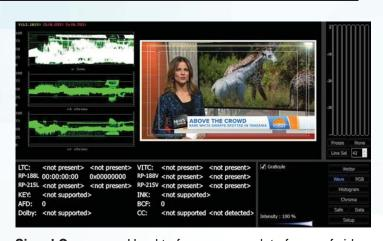
**Signal Compare** - Used to freeze a complete frame of video (two fields in interlaced), every second line (field) or at a 50/50 dissolve to compare two signals or cameras.
