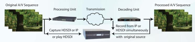
2) Send a known sequence via SDI to the processing unit, record the output from a hardware decoder and compare this to a pre-recorded result - generating pass fail to a ClearView log file or CLI script.
