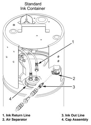
*Figure 6-7. Flushing the ADS*
