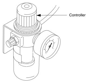
Figure 4-2: Air Regulator on One Litre Fluid System
