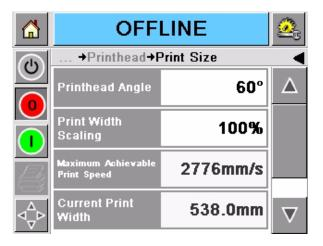
Figure 4-17: Select Printhead Angle
