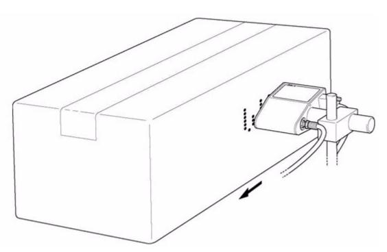
Figure 5-15: Message Printed Late (800 Series Printhead)
