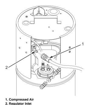
Figure 4-6. Removing Air from the Ink System
