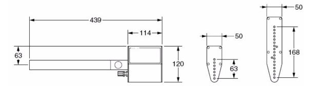
Figure A-3. 800 Printhead Dimensions (mm)
