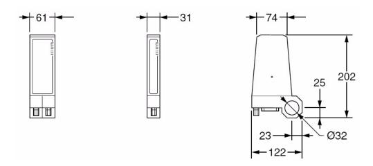
Figure A-2. 700 Printhead Dimensions (mm)
