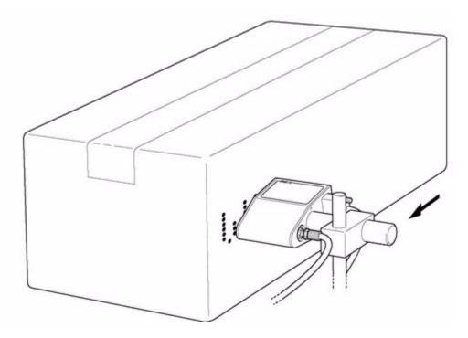
Figure 5-14: Message Printed Early (800 Series Printhead)
