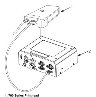
Figure 1-1: Videojet 2120 Printer with 700 Series Printhead
