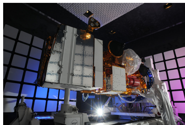
Caption: Electromagnetic compatibility testing occurs inside a specially designed room that stops the reflection of sound or electromagnetic radiation, called an anechoic chamber.
