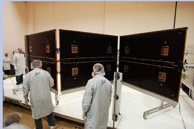
Caption: On a slick floor made of polymer roofing material, NPP's solar panels glide on a cushion of air to test the mechanisms that unfold and lock the solar array into place.
