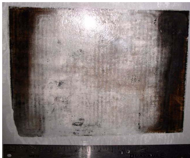
Figure 2. Close-Up of End-of-Life Membrane Showing Potential Contamination in the Membrane at Reactant Gas Inlets
