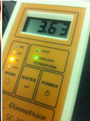
Figure 14. Make sure that the green "PROCEED" LED is lit. You should be reading a pH close to what you expect your wine is at.
