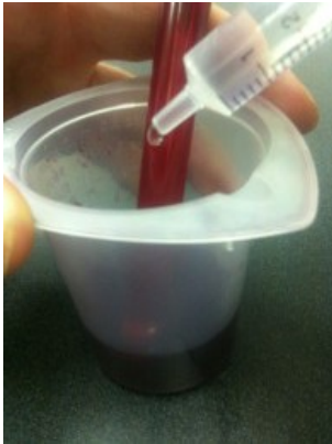
Figure 12. Manual stirring technique. Hold the electrode against the side of the titration beaker and swirl gently; add TA Titrant with other hand.
