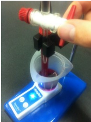
Figure 13. Automated stirring technique. Turn on the magnetic stirrer; add TA Titrant by slowly opening the burette stopcock valve.
