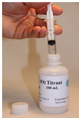
Figure 5. Withdraw the titrant from its bottle using a clean 5 mL syringe. If you are using the glass burette, use the syringe to fill it.
