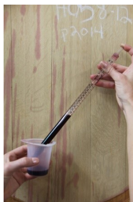
Figure 6. Dispense 25 mL of your wine into the titration beaker using the 25 mL sampling pipette. Make sure this is clean before putting the pipette into your wine container!
