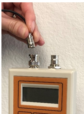
Figure 2. Attach the SO 2 electrode to the connector on the SC-300.
