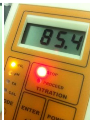
Figure 11. Once the device beeps for 15 seconds or 20 sets of "beep-beep", you are done with the titration. The red "STOP" LED will also remain lit.
