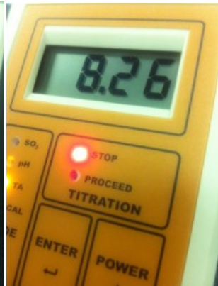
Figure 15. Once the pH arrives at or passes 8.20 you are done with the titration. The red "STOP" LED will be lit and the instrument will be beeping
