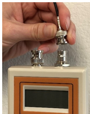
Figure 3. Be sure the pH electrode attachment is screwed into place on the BNC connector.
