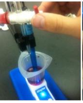
Figure 18. Automated stirring technique. Turn on the magnetic stirrer; add SO2 Titrant by slowly opening the burette stopcock valve.
