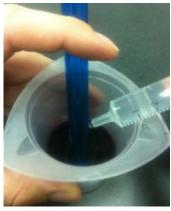
Figure 17. Manual stirring technique. Hold the electrode against the side of the titration beaker and swirl gently; add SO2 Titrant with other hand.
