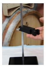
**Figure 5.** The Electrode Holder slides onto the Lab Support Stand.
