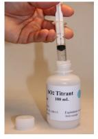
Figure 14. Withdraw the titrant from its bottle using a clean 5 mL syringe. If you are using the glass burette, use the syringe to fill it.
