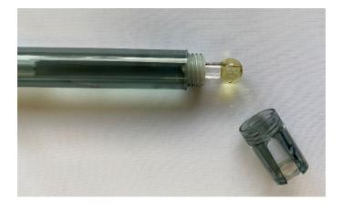
3. They have a porous ceramic frit for a reference junction. The earlier models used a polymeric material. This does not require any additional attention on your part, but we found that this reference junction is less affected by lack of stirring, and the pH accuracy below pH 3.2 is slightly improved.
