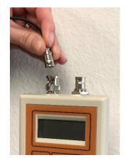
**Figure 2.** Attach the SO2 electrode to the connector on the SC-300.
