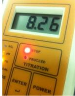
Figure 24. Once the pH arrives at or passes 8.20 you are done with the titration. The red "STOP" LED will be lit and the instrument will be beeping
