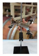
Figure 7. The Double Burette Clamp slides easily onto the Lab Support Stand.
