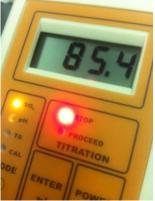
Figure 20. Once the device beeps for 15 seconds or 20 sets of "beep-beep" you are done with the titration. The red "STOP" LED will also remain lit.
