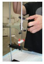
Figure 8. The burette sits firmly between the notches of the four spring arm knobs of the Double Burette Clamp.
