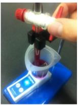
Figure 22. Automated stirring technique. Turn on the magnetic stirrer; add TA Titrant by slowly opening the burette stopcock valve.
