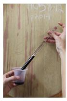
Figure 15. Dispense 25 mL of your wine into the titration beaker using the 25 mL sampling pipette. Make sure this is clean before putting the pipette into your wine container!
