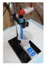
Figure 4. The Magnetic stirrer and beaker with the pH electrode inserted into the Electrode Holder to the wine sample.
