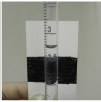
Figure 13. Reading the meniscus of the water column is easier and more precise if you use the paper with the black band held up an inch behind the burette and its black band 1/2 an inch below the meniscus. In this picture the value from Figure 11 is further resolved to 3.26 mL.
