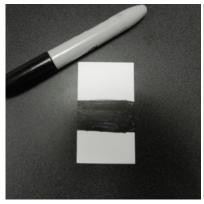
Figure 11. On a thick white sheet of paper or a business card, use a black marker to draw a band approximately an inch and a half thick. This card will assist you in reading the burette accurately.
