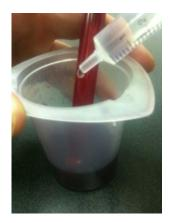
Figure 21. Manual stirring technique. Hold the electrode against the side of the titration beaker and swirl gently; add TA Titrant with other hand.
