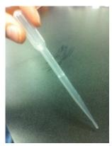
**Figure 16.** The transfer pipette. One full squeeze of the transfer pipette in either the Acid solution or Reactant should be approximately 2 mL.
