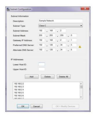
The form shown below now reflects the % ample Network+added in the previous steps. The IP addresses defined in this network will now be available to assign to the Valcom devices and will be scanned when % can using current network settings+is selected.
