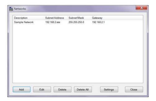
Click the **Close** button to close this dialog box. To scan the network for Valcom devices using this newly-defined network, click the Communications menu on the main application screen, then choose Scan All Devices.
