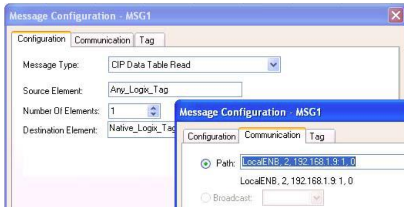
Figure 98 – Message Configuration » Configuration and » Communication tabs in PLC setup utility
