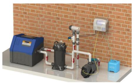
The Chlorine Sensor uses Oxidisation Reduction Potential readings to determine the chlorine level in your pool or spa water.
