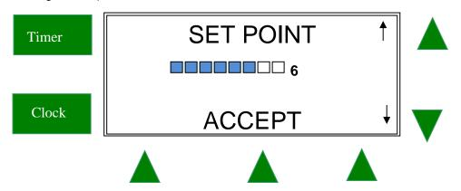
Use the up and down buttons to change the Set Point between o and 8. o chlorine output should only be used when there is no salt in the water. In summer, the chlorine should be set between 6 and 8 and you should regularly check your chlorine level in your swimming pool to determine if the output should be increased or decreased. Rely on your pool professional for advice on the recommended chlorine level in your pool.
