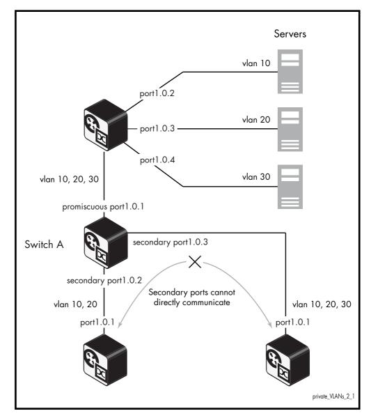
The ports on **Switch A** have the following configuration:
