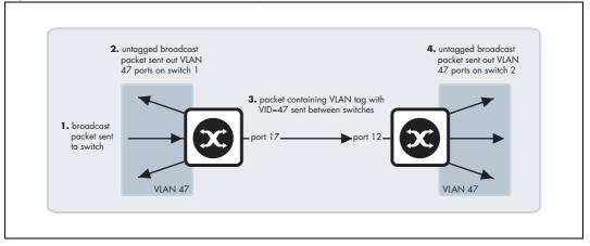
The tag makes it very easy for the second switch to know what to do with the packet, because the tag marks this packet as belonging to VLAN 47, and switch 2 knows exactly what it should do with packets that belong to VLAN 47.
