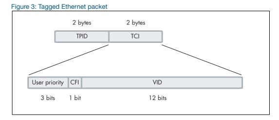
**TPID** is the tag protocol identifier, which indicates that a tag header is following and contains the user priority, Canonical Format Indicator (CFI), and the VLAN ID.
