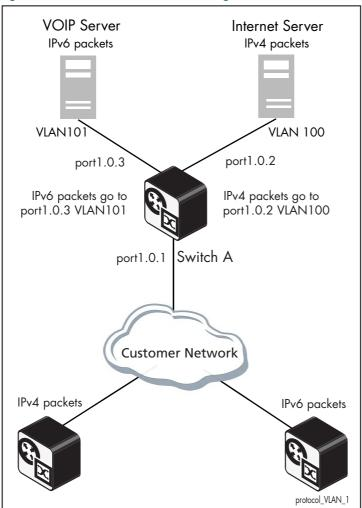
Figure 13: Protocol based VLAN configuration
